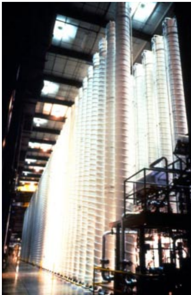
Figure 21. Gas Centrifuge Cascades at ORGDP. Photograph circa 1978.
