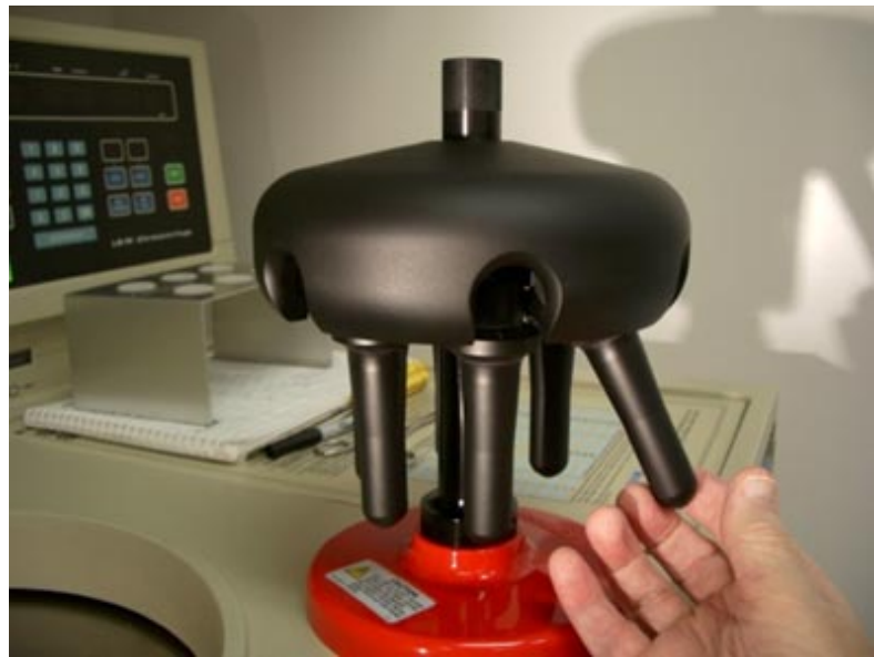
Figure 5. Contemporary Swinging Bucket Rotor (Beckman SW41 Ti). Maximum Speed: 41,000 rpm, Maximum Centrifugal force: 288,000 x g, Maximum Volume: 79.2 ml, Number of Tubes: 6
