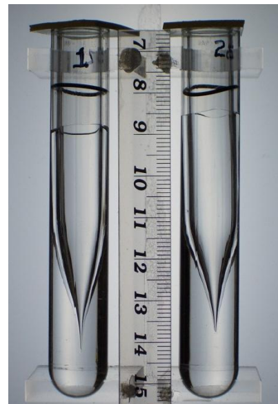
Figure 3. Glass Heat-Drawn Micro-banding Tubes Floating in 0.8 RT Saturated CsCl in Beckman SW 41 Rotor Tubes. Scale Indicates Distance from the Center of Rotation.
