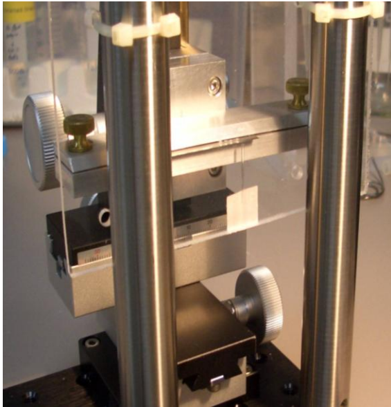
Figure 18. Microtome (Viratome) for Sectioning Microbanding Tubes
