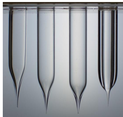
Figure 2. Microbanding Tubes Heat Drawn to Obtain a Sharp Internal point.
