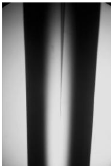
Figure 5. Borosilicate Glass Microbanding Tube Drawn to a Sharp Internal Point.
